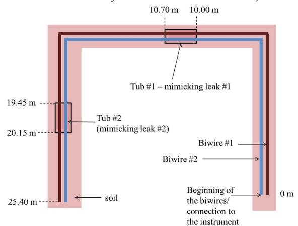
Fig. 2 Schematization of the layout of the experimental apparatus.
