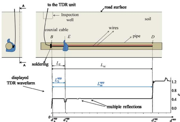
Fig. 1 Schematization of the typical layout of an underground pipe equipped with the distributed biwire. The figure below shows a schematization of a typical reflectogram in presence of a leak.
