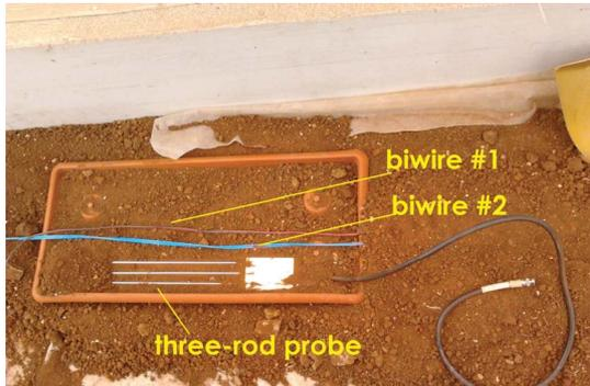
Fig. 3 Tub placed at 10.00 m from the beginning of the biwires. The soil inside the tub was progressively moistened with increasing amount of water. A three-rod probe was used to monitor the moisture content of the soil inside the tub.
