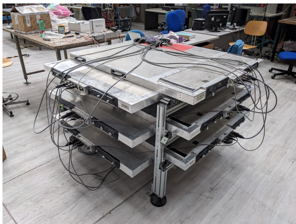
Figure 1. View of the MURAY detector setup used during tests and electronics upgrade. Each plane consists of two orthogonal layers read out by SiPM-based front-end boards.
