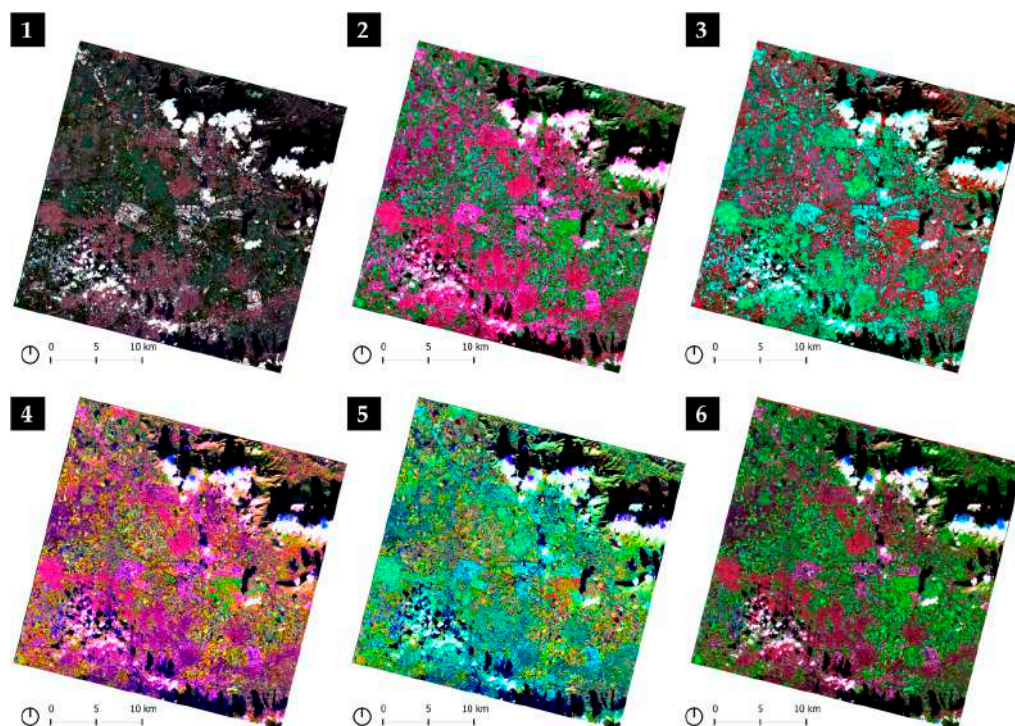
Figure 6. Maps resulting from false-color combination: 1—natural color; 2—false color; 3—color infrared; 4—agriculture; 5—healthy vegetation; 6—recent harvest.
