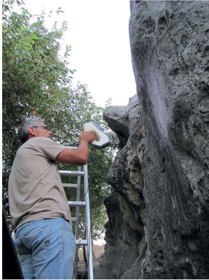
Fig. 9: Detailed surveys using structured light scanner Art Eva (Photo: M. Marazzi, 2017).
