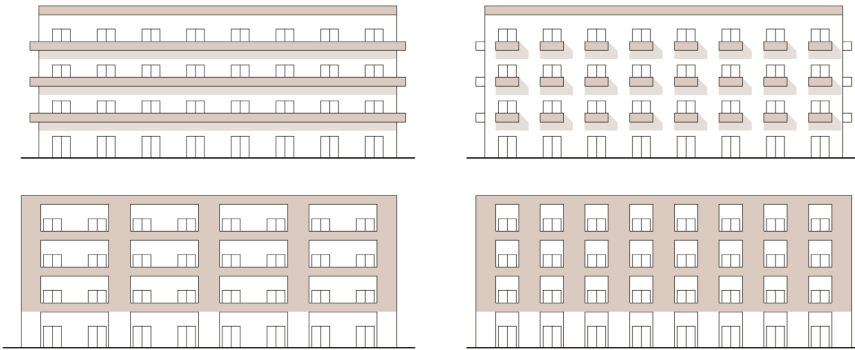
Fig. 5. Suitable areas (in red) for PV integration. on balconies (top) and loggias (bottom).
