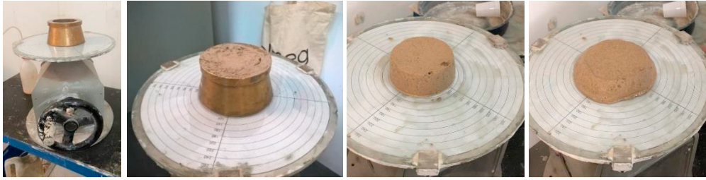
Fig. 1. Workability test on hemp plasters.
