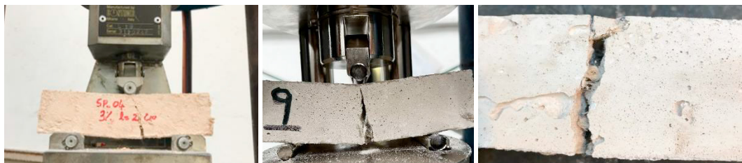
Fig. 5. Sewing effect of hemp fibres in the three-points bending test.
