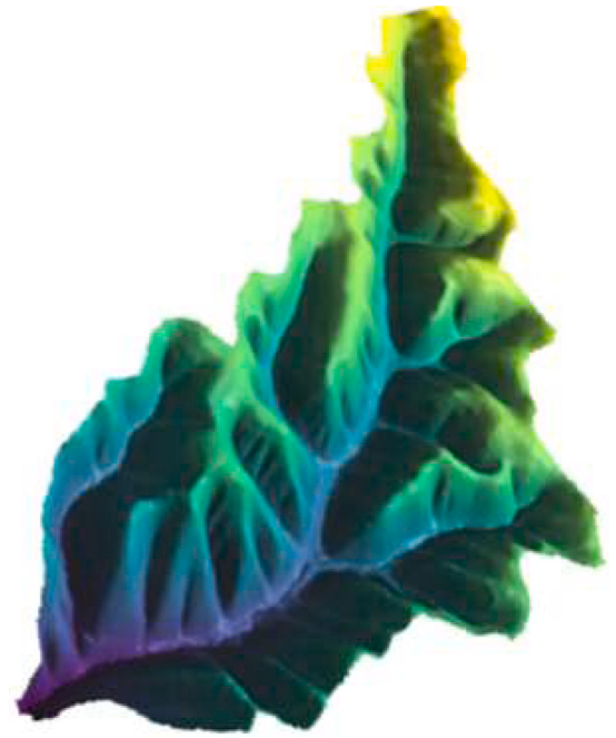
Fig. 3. Digital Elevation Model (DEM) of the basin near the city of Mesa in the State of California (USA). This DEM is obtained using the LiDAR optical sensor technology, with a resolution of 1 \text{ m} \times 1 \text{ m} .
