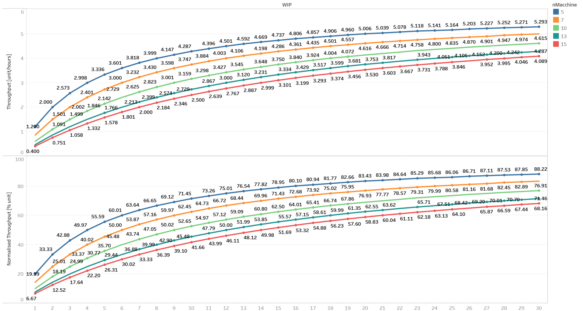
Figure 6. The throughput and normalized throughput when varying the number of machines (in different colors) with alpha value fixed at 1 and mean processing time fixed to 10.
