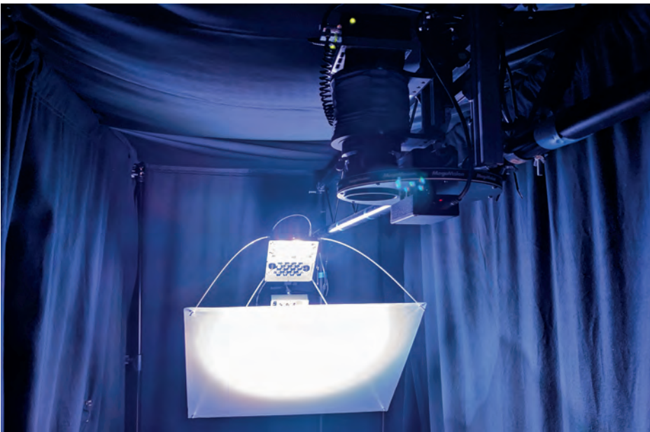
Fig. 2. Multispectral imaging system: UV-IR LED light panels
