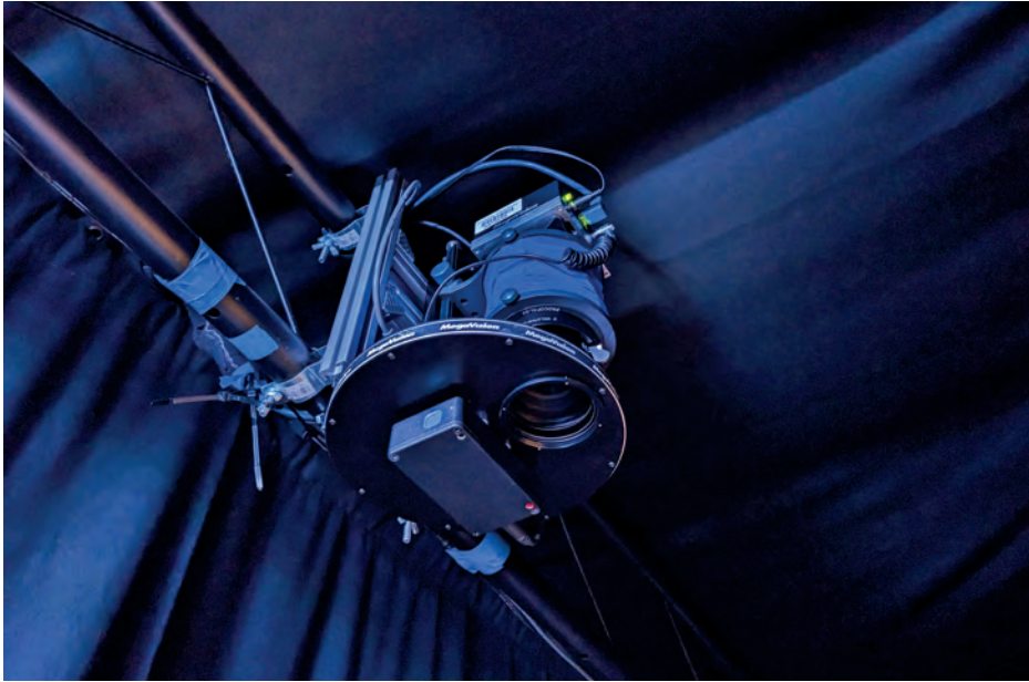
Fig. 1. Multispectral imaging system: 50 megapixel E7 camera back
