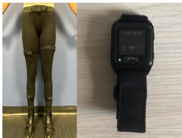
Figure 7. On the left, classic positioning of wearable sensors on the lower limbs to calculate joint kinematics is shown; on the right, an example of the wearable sensor APDM Opal™ ( https://share.apdm.com/documentation/MobilityLabv1UserGuide.pdf (accessed on 4 April 2024), APDM, Portland, OR, USA), which is composed of two accelerometers, one gyroscope, and one magnetometer that records in three axes (vertical, mediolateral, anteroposterior), is shown.
