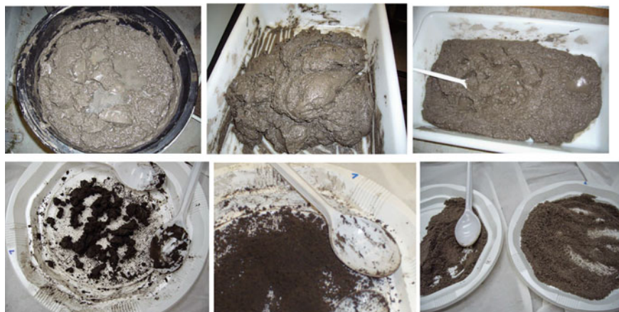
Fig. 4 Some raw (up) and treated (down) sewage sludge samples used by the authors of the book
