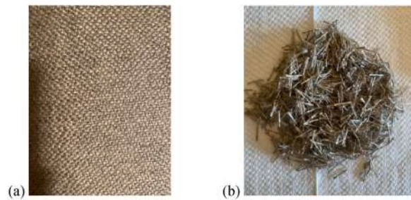
Fig. 1. Hemp fabric (a) and cut hemp fibres (b).
