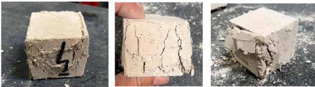
Fig. 9. Specimens after compressive strength.
