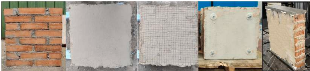
Fig. 14. Manufacturing phases of the reinforced wall (Reinf_01) and regularization of the end cross-sections.
