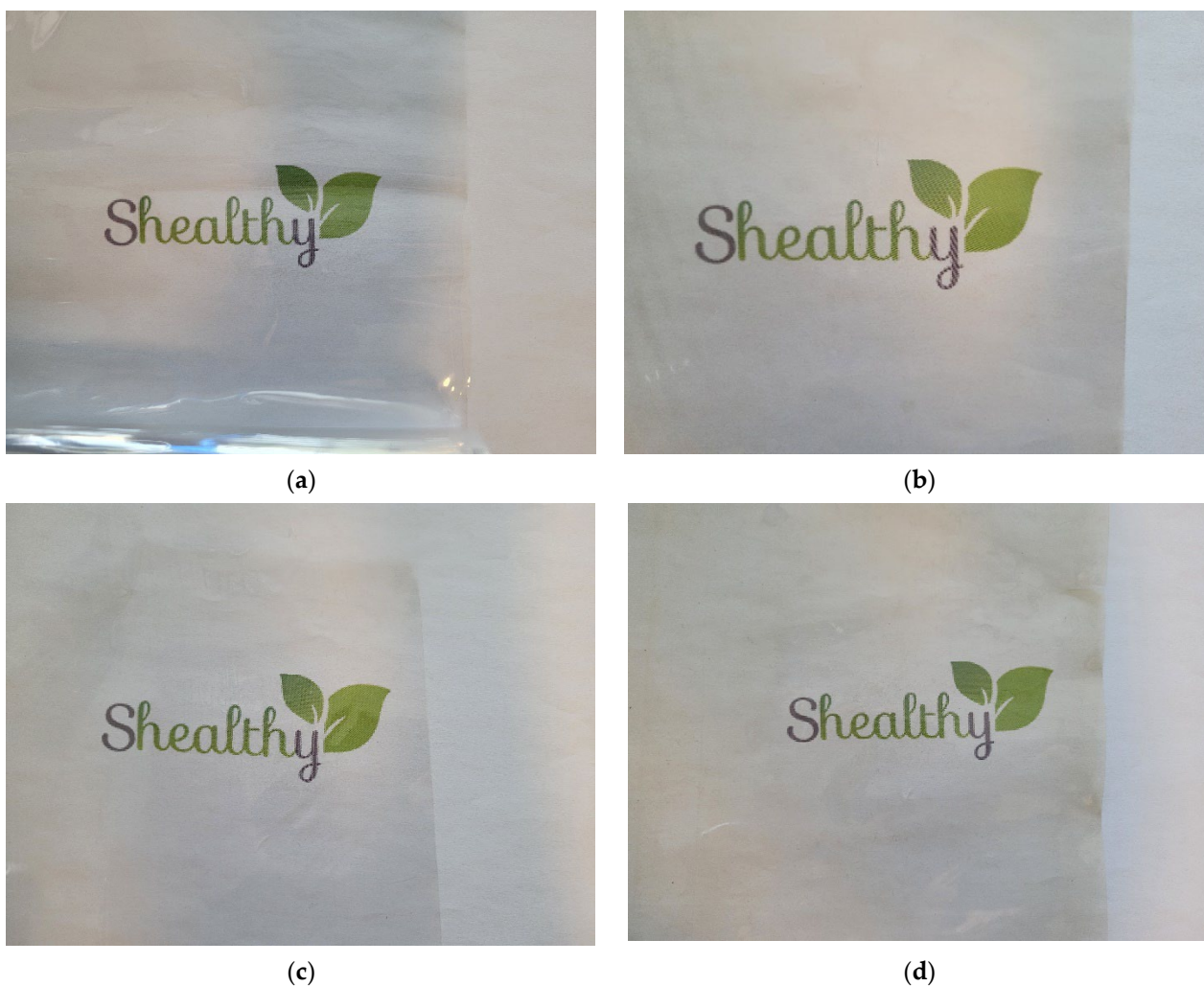
Figure 1. Images of the active films processed at a semi-industrial scale: (a) polypropylene (PP); (b) polypropylene + orange peel extract (PP + OPE); (c) polylactic acid (PLA); (d) polylactic acid + orange peel extract (PLA + OPE).
