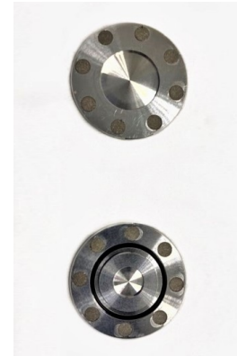
Figure 2. The front and the back part of the coin target (24 mm diameter, 2 mm thick).
