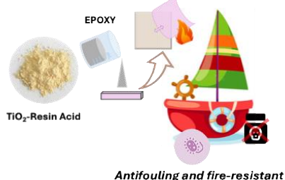
Figure 1. Antifouling and fire-resistant epoxy composite coatings via rosin–TiO 2 hybrid particles.
