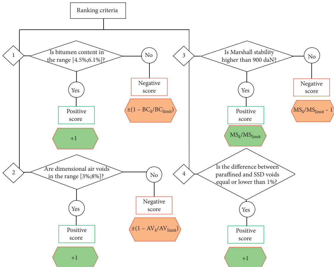
FIGURE 13: Flow diagram of the ranking procedure and ranking criteria.
