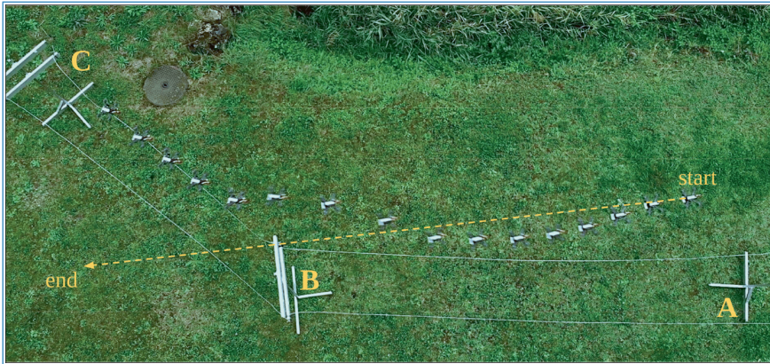
Figure 8.1. A quadrotor performing power line inspection in a power line test environment with three masts (labelled: A, B, and C) using our proposed approach. The original rough reference trajectory is depicted in yellow and the drone deviates from it while avoiding obstacles (the power masts) and keeping the power line visible in the field of view of the onboard camera.
