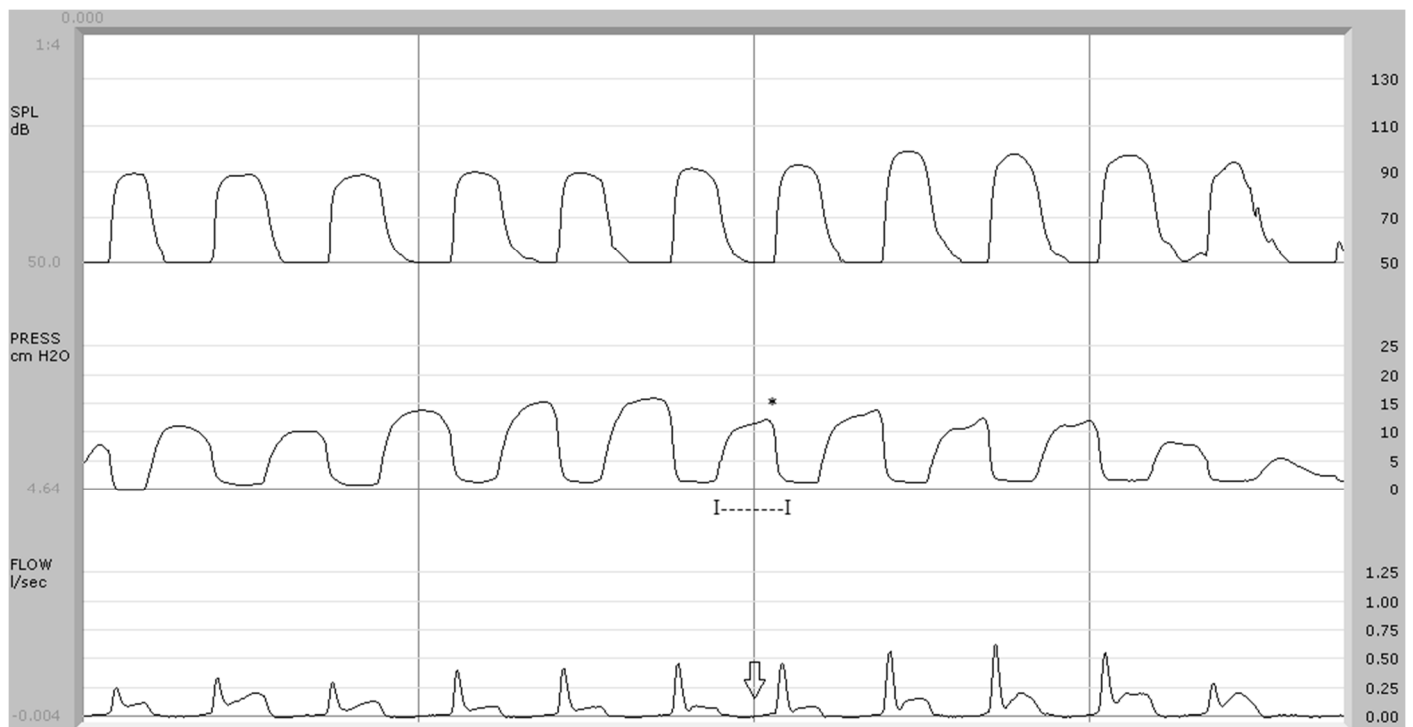
Figure 4. Syndromic patient (case no. 8). In the center trace, the average pressure peak (*) is 14.2 cm H 2 O and the pressure duration is 194 msec (I—I). Below, the arrow indicates the absence of airflow during the implosive phase of /p/. Discriminant analysis classified this subject as “borderline” (discriminant score: -0.011 ).
