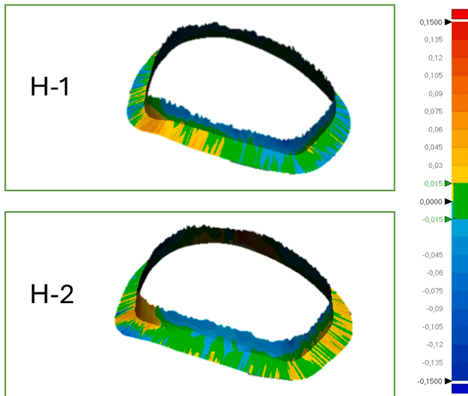
Fig. 5. Marginal trueness after the best-fit alignment. Green regions denote the least displacement of the experimental scans relative to the reference model.
