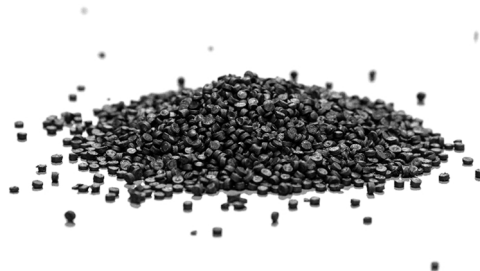
Fig. 1. The Graphene-enhanced recycled plastic (GRP) asphalt modifier.
