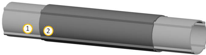
Figure 4. Sketch of two segments joined with collar; 1-radius = 80 mm; 2-radius = 86 mm.
