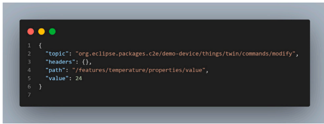
Fig. 11. Cloud2Edge command expressed in JSON format.
