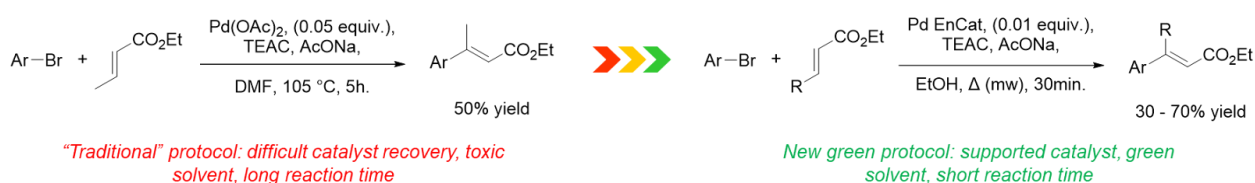
Figure 1: Comparison between the old and new protocol for the Heck reaction.
