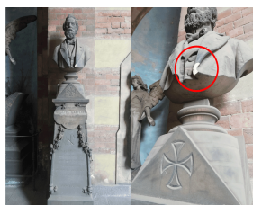
Figure 1: Funerary monument. The red circle indicates the black crust detachment.
