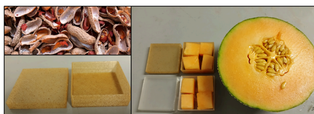
Figure 1: Bio-packaging boxes incorporating peanut shell powder for fresh fruit preservation.
