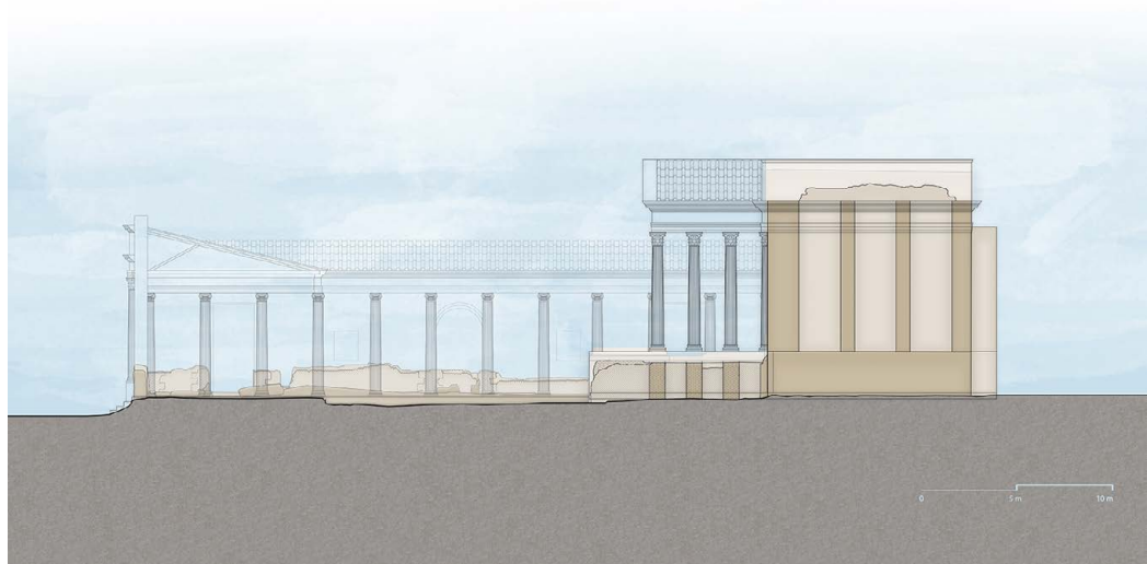
Fig. 9. Longitudinal section with reconstruction of the Temple of Divus Vespasianus in Cuma. Elaboration by Alessandra Pagliano.
