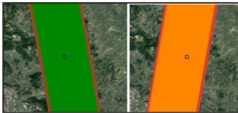
Figure 3. Tracks of SAR images used in the area of interest (indicated in the black square) available in the ASI archive: ascending mode (left), descending mode (right).
