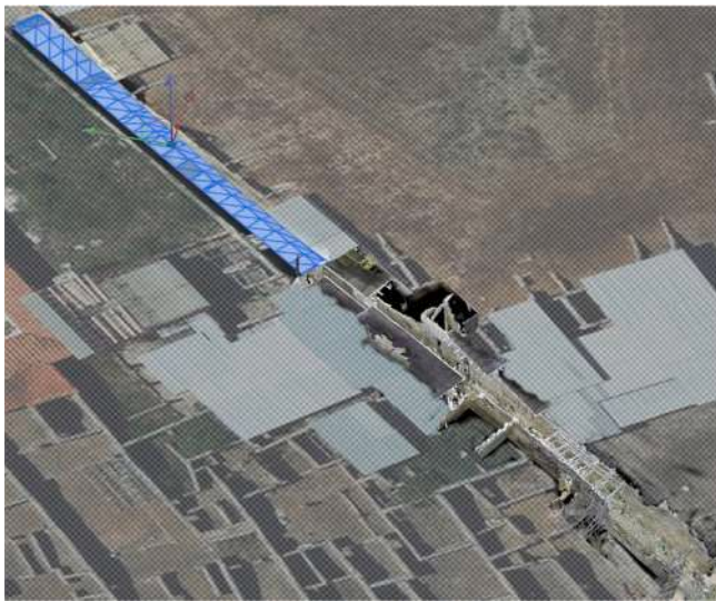
Fig. 9. Model view: selection of the parametric object is edged in blue colour; the southern part of the alley is represented by the point cloud; the topographic background is made available from BING maps.
