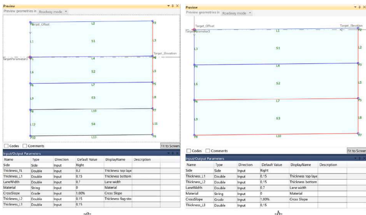
Fig. 8. Assemblies overview in Subassembly composer with some parameters: (a) Paved stretch cross-section; (b) Unpaved stretch cross section.
