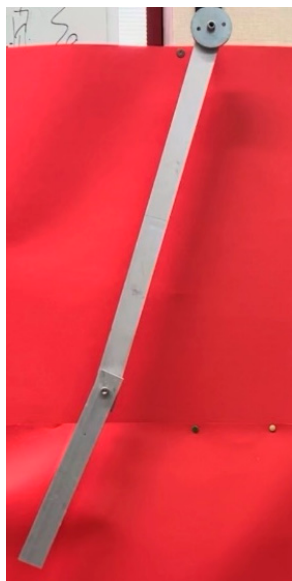
Figure 2. Double pendulum used for the measurements in Tracker. Length of the longer bar is L_1 = 0.66 m, length of shorter bar is L_2 = 0.33 m, total mass is M = 3 kg.
