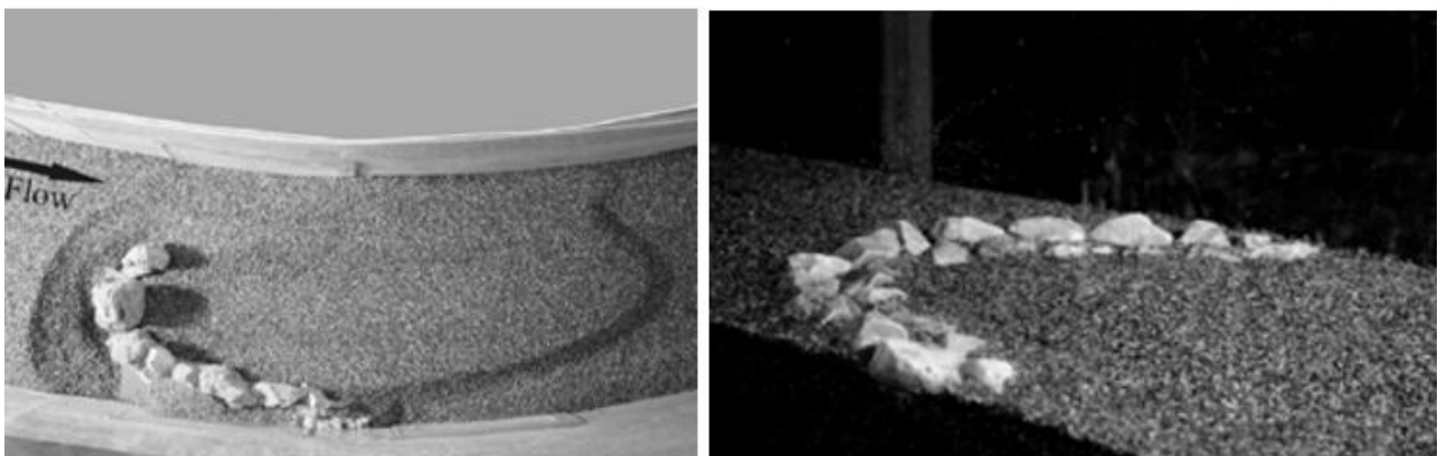
J-hook in a curved channel (left) and cross vane in a straight channel (right), inserted in a river bed (experiments conducted in physical models – University of Pisa)
