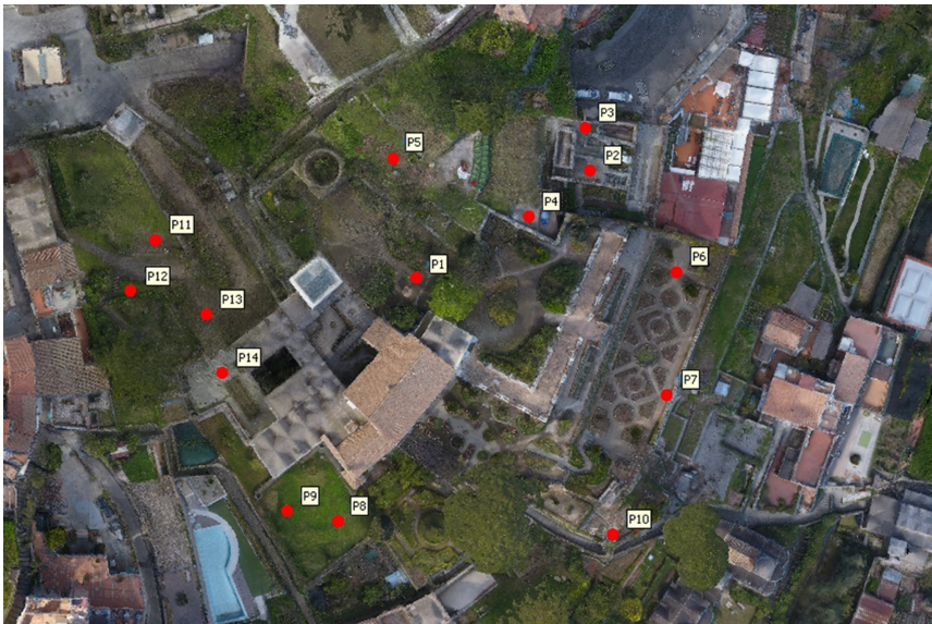
Fig. 4. Orthophoto showing the homogeneous distribution of the 14 GCPs, with an elevation difference between P4 and P9 of about 19 meters (by Marco Limongiello).
