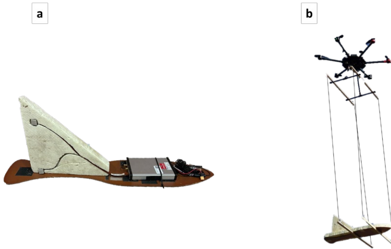
Fig. 1. MFAM configurations used for the surveys. a) Geometrics MFAM “Development kit” arrangement inside the prototype bird with the additional frame which allows distancing of the sensors; b) UAV flight configuration.
