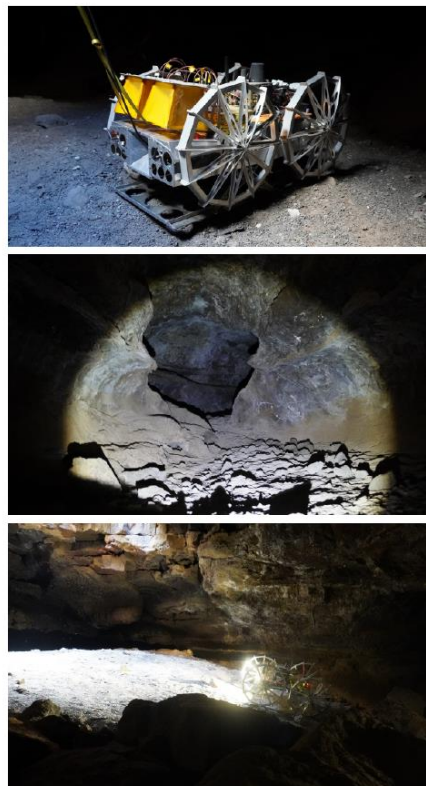
Figure 4: Shows the end of MP3 and beginning of MP4, where Coyote3 reaches the ground of the lava tube, undocks from the TMDS and starts exploring the cave (credit: DFKI, Meltem Fischer).
