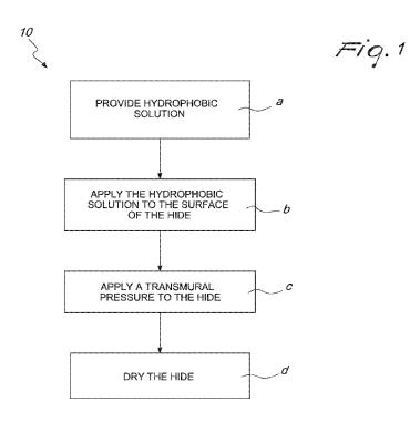
(57) **Abstract:** A functionalizing treatment method for hides and the like that have a surface and an internal substrate that comprises interconnected fibers, which comprises a deposition step (10), in which a plurality of functionalizing elements comprising nanomolecules and/or nanoparticles are inserted into the internal substrate of the hide to be treated, between the individual fibers, so as to coat and functionalize the individual fibers.
