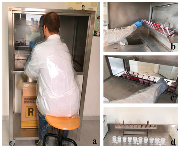
Fig. 3. EchinoHood. (a) Laboratory technician while working under the EchinoHood; (b) Aliquotation of 10 fresh faecal samples using the Fill-FLOTAC collectors; (c) Removal of the support with the Fill-FLOTAC after aliquoting of the faecal samples; (d) 10 fresh faecal samples ready to be processed.
