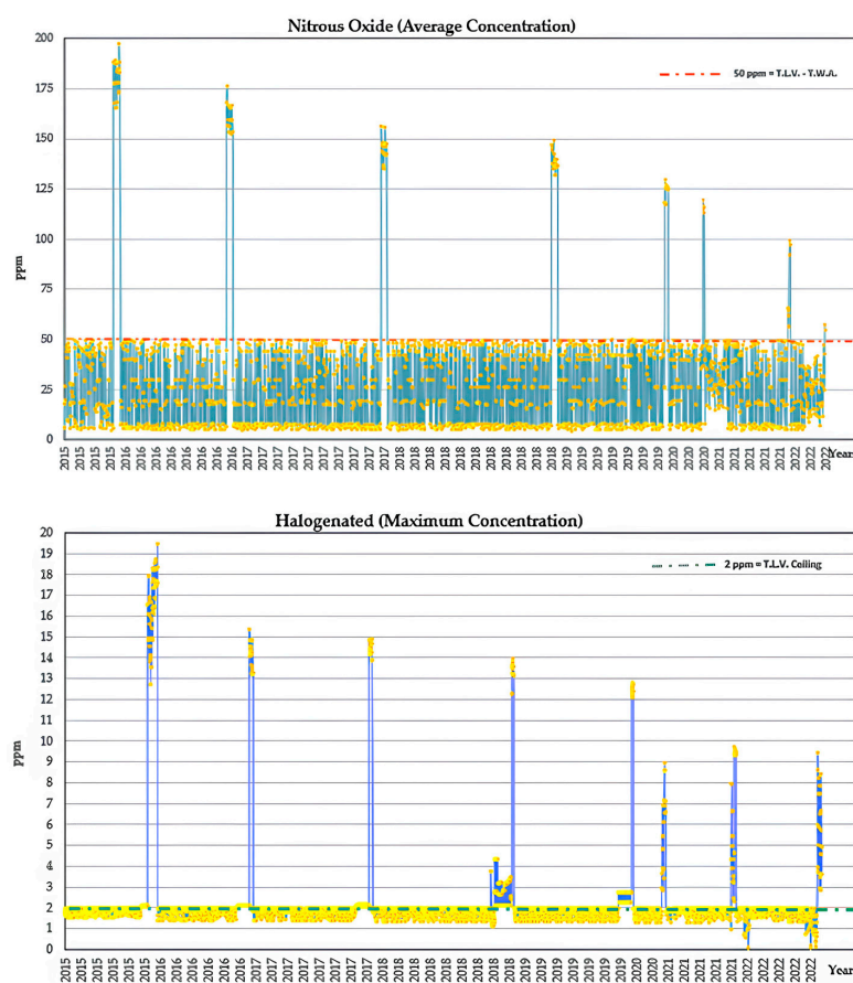
Figure 5. Concentration of Halogenated gases and nitrous oxide from monitoring conducted during the study years 2015–2022.
