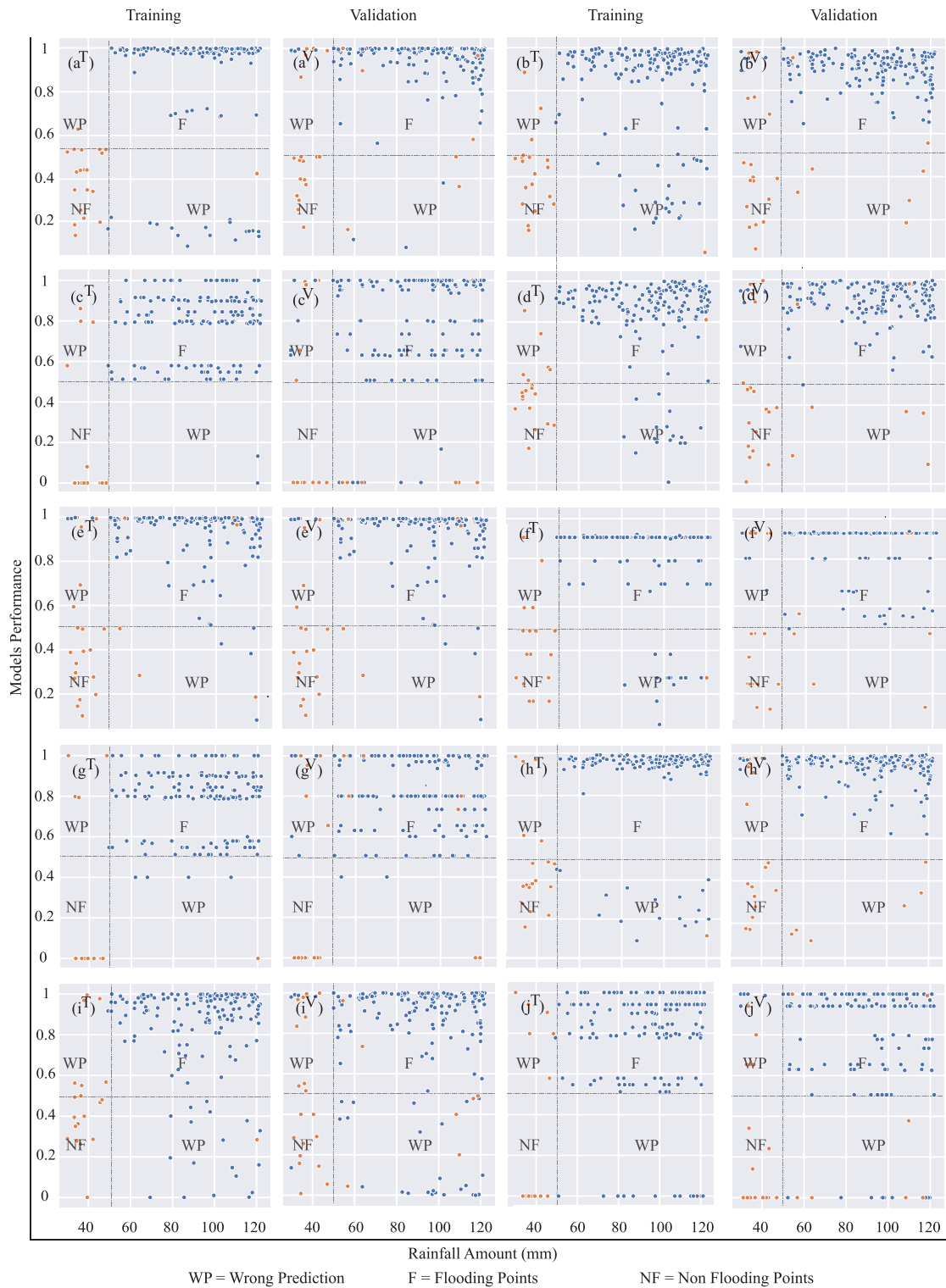
Fig. 9. Performance of all ML models during the training and validation (a) LightGBM, (b) RF, (c) NN's, (d) LG, (e) XGBoost, (f) SVM, (g) KNN, (h) CBC, (i) NB and (j) DT.
