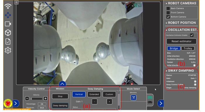
Fig. 2. CERN Human Robot Interface showing the sway damping control integration with the following elements on the scene: (a) The control panel, (b) The oscillation estimator status feedback messages, and (c) The sway damping status feedback messages.
