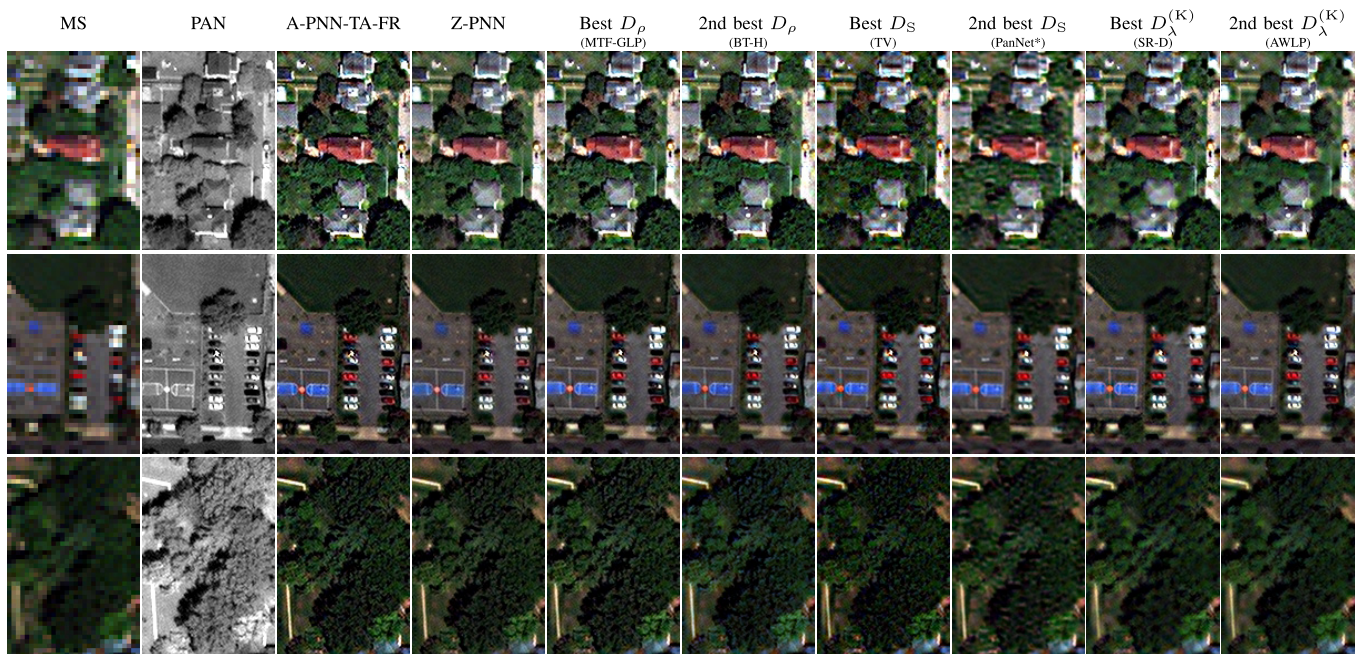
Fig. 14. Results for some WV2 crops. (From Left to right) MS, PAN, A-PNN-TA-FR, and Z-PNN, best references for D_\rho , D_S , and D_\lambda^{(K)} .
