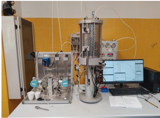
Fig 3. Double-walled unsaturated stress path (USPv2), University of Naples Federico II.
