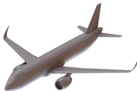
Fig. 5 Render of the 3D model of the baseline aircraft, automatically generated with JPAD.
