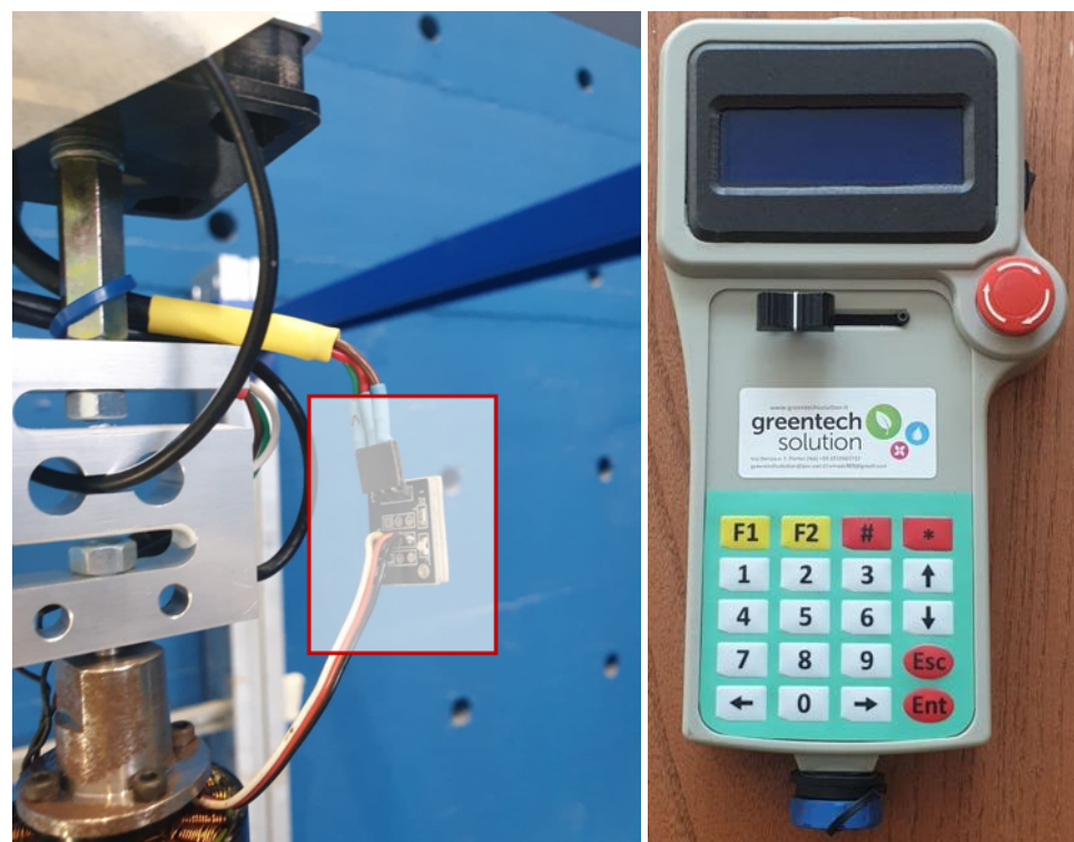
Figure 5. Magnetic Hall effect sensor (left) and handheld computer (right).
