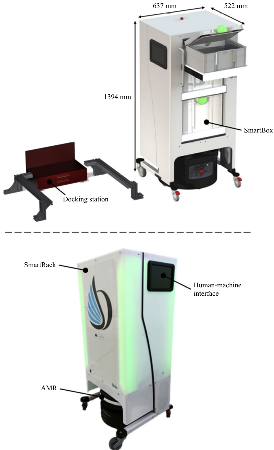
Figure 1. Design of the HOSBOT, an autonomous mobile robot system, utilized in this study for hospital logistics and disinfection evaluations. Top: Front view of the HOSBOT and its docking station. SmartBoxes can be retrieved from the SmartRack upon authorization. Bottom: Photograph of the HOSBOT navigating an obstacle-free environment, with green LEDs illuminated. The human–machine interface is accessible via a tablet located on one side of the SmartRack.
