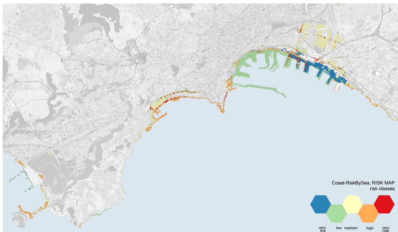
Figure 5. Coast-RiskBySea on Naples (Italy), risk map to ESL (RCP 8.5, 100 yr RP, 95%). Source: [41].
