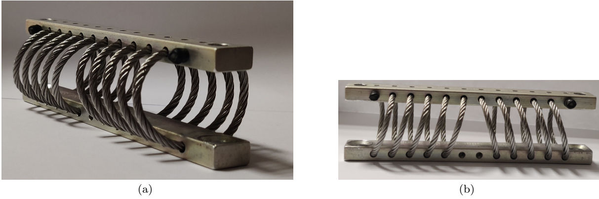
Fig. 1 Helical wire rope isolator: (a) tested device and (b) its shear direction.
