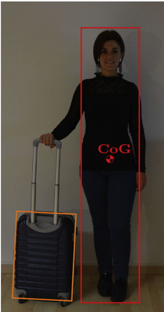
Fig. 4. Shape detection of passenger and luggage.
