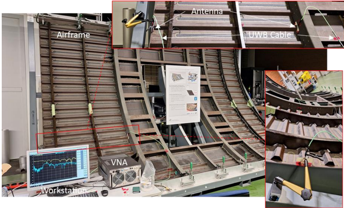
Fig. 2. Experimental setup for UWB microwave leakage monitoring aiming at stringer debonding assessment on the large-scale fuselage segment. The enlarged pictures highlight the placement of the antenna.
