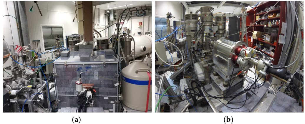
Figure 8. The two experimental setups used in the LUNA campaigns on the ^{22}\text{Ne}(p, \gamma)^{23}\text{Na} reaction. (a) Setup used during the HPGe campaign. The Dewars of the two HPGe detectors are visible, close to the lead shielding and the radon box. (b) Setup used during the BGO campaign. The beamline is passing through the segmented BGO detector, that is standing unshielded.
