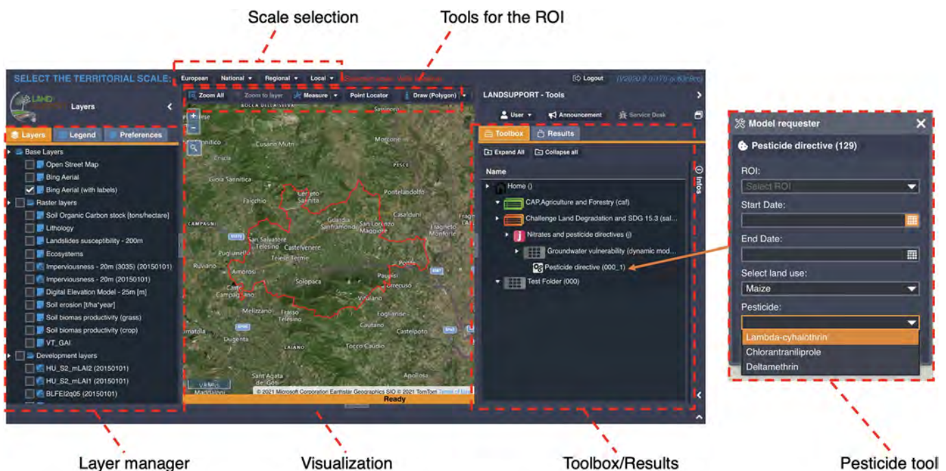
Fig. 2. Five sections can be distinguished within the LS dashboard: i) the scale selection, ii) the tools for the ROI, iii) the toolbox/results, iv) the layer visualization and v) layer management. The pesticide fate tool panel consists of five entries: the ROI, the start and end dates of simulation, the crop and pesticide selections.
