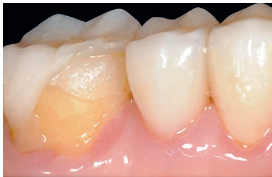
▲ Fig 7 Ceramic fracture on a mandibular first molar. The restoration had an occlusal thickness of about 1 mm and was cemented onto a substrate with a prevalence of dentin.
