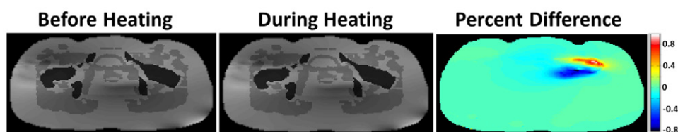
Figure 3. Simulated proton density weighted gradient echo images before and during focal heating, and the percent difference between them.
