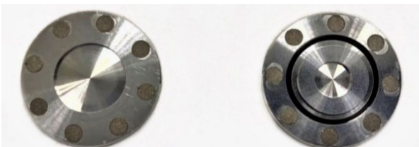
Fig. 3. The front and the back parts of the coin target (24 mm diameter, 2 mm thick).
